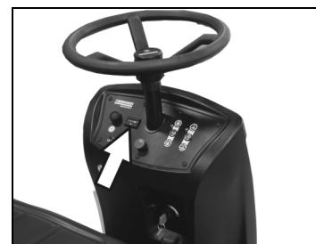
Elapsed-time meter indicates maintenance interval times.
